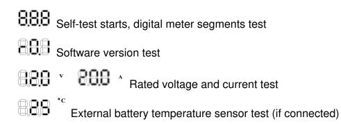
After going into charging process, the LCD displays the charging statues as below: Press **VOLT** / **AMP button** in sequence, the LCD will display in turn with Battery Voltage, Charging Current, Charged capacity (Amp-hour) and Battery Temperature (if external temperature sensor connected)
