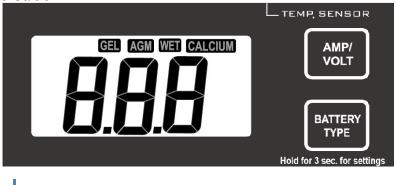
Press **BATTERY TYPE button** and hold for 3 seconds to go into your battery type selection mode, the battery type you select will be shown on the LCD meter, the default setting is AGM Battery; the controller will automatically memorize your battery type setting.
