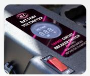
Monitor the voltage of your battery at any-time & identify when it may be running flat
