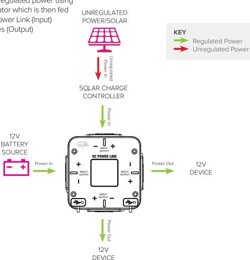
Reccommended Suggestions: Selected suitable Amperage Solar Controller based on your single 12V Solar Panel. It is recommended that suitable fuses are placed on the positive cable to devices chosen and also between Solar Panel Positive to the Solar Controller selected.
