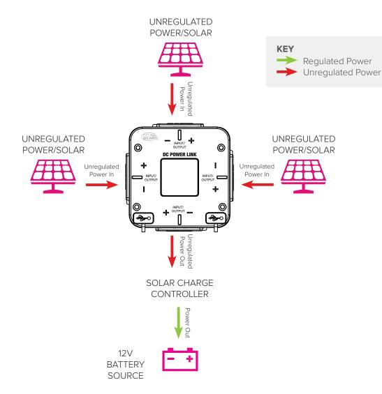
Tip: As you are fitting 3 panels in parallel configuration, the Amperages are therefore tripled. If fitting 2 panels, the Amperages are doubled. Select the correct Solar Charge Controller Amperage. We recommend suitable fuses are placed on the positive cable to devices chosen and also between Solar Panel Positive to the Solar Controller selected.
